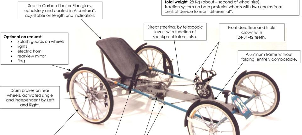
Rear wheels (Aluminum rim) with tires inner tube, customizable 16", 20" or 24".
